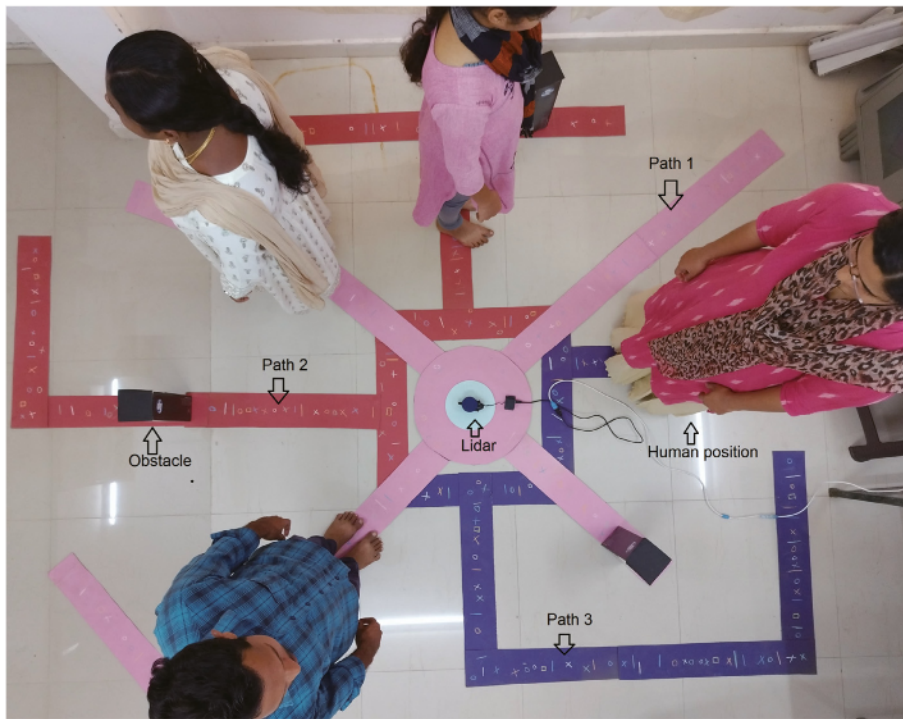
Fig. 11. Experimental setup of LiDAR data collection for Scenario II, whereby the LiDAR was placed in the middle of the closed environment with multiple objects. Three different color strips are used to indicate the path of the people moving about in various instances.
