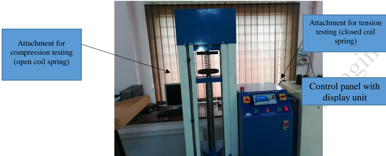
Figure 5.1 Experimental setup with open coil spring
