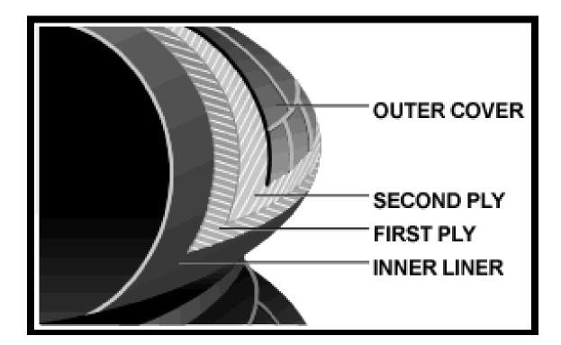
A standard two ply air spring is actually made up of four layers.
