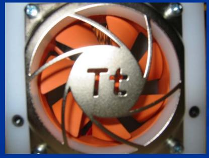
Air would be blown by twin fans across the heat sinks removing excess heat
