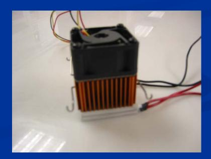
Refrigeration compartment would be atop the Thermoelectric modules while fans would cool the heat sinks.
